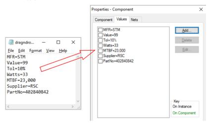
Note: Copy Paste does not work for this function, the text must first be selected, then dragged to the appropriate Easy-PC dialog.
