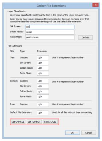
Extension Side Type Extension Extension Top: Copper: .top .cmp .qtl Silk Screen: .plc .sst .gto Solder Resist: .stc .smt .gts Paste Mask: .pmc .spt .gtp Bottom: Copper: .sol .bot .abl Silk Screen: .pls .ssb .gbo Solder Resist: .sts .smb .gbs Paste Mask: .pms .spb .gbp Inner: Copper: .g# .gbr .g# Default File Extension: .gbr .gbr .gbr
