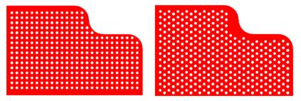
The picture above shows both Normal via distribution and Staggered.
