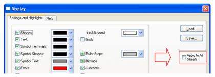
When checked, the colours displayed for the active schematic design will be applied to all other schematic designs in the project when **OK** or **Apply** are clicked. This includes nets colours for nets present in the active design.
