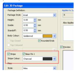
**CAN** shapes will get a stripe up the side of the body near to pin 1 or pin 2 depending on the pin 1 checkbox. **Axial** components get a single stripe near one end or the other (Capacitors, Diodes etc.), except for **Resistors** (R) and **Inductors** (L) which will get the correct set of coloured stripes depending on the value of each component. The **Value** attribute is read and converted to a standard colour coding. Values in formats such as 2.2K or 2K2 are accepted and converted.
